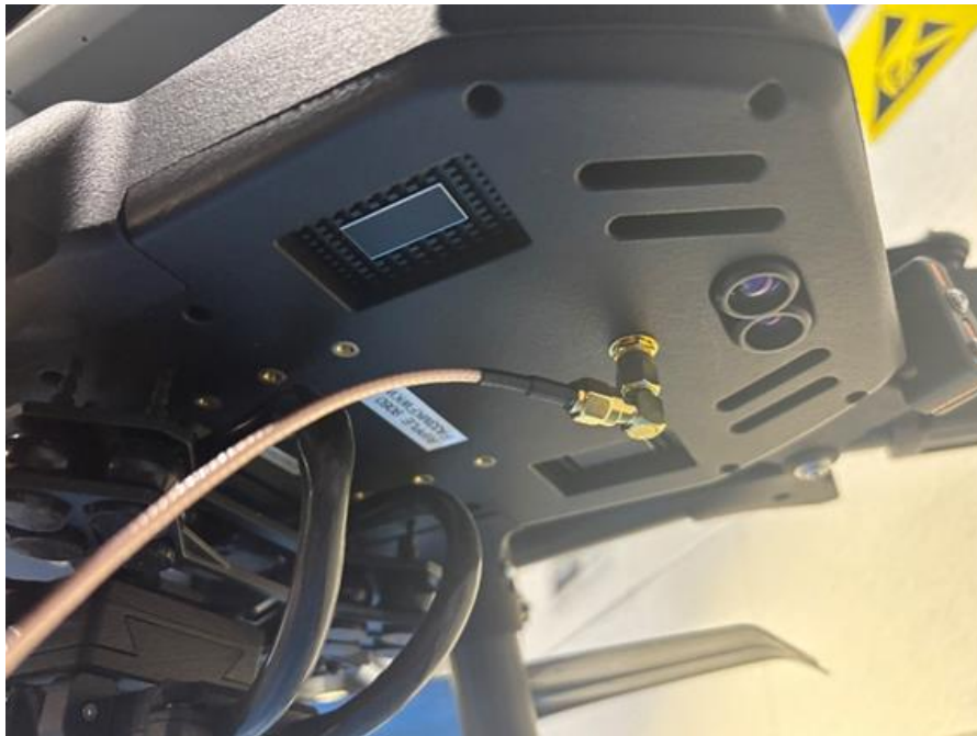
Figure 5-11: GNSS cable connected to the IF800
