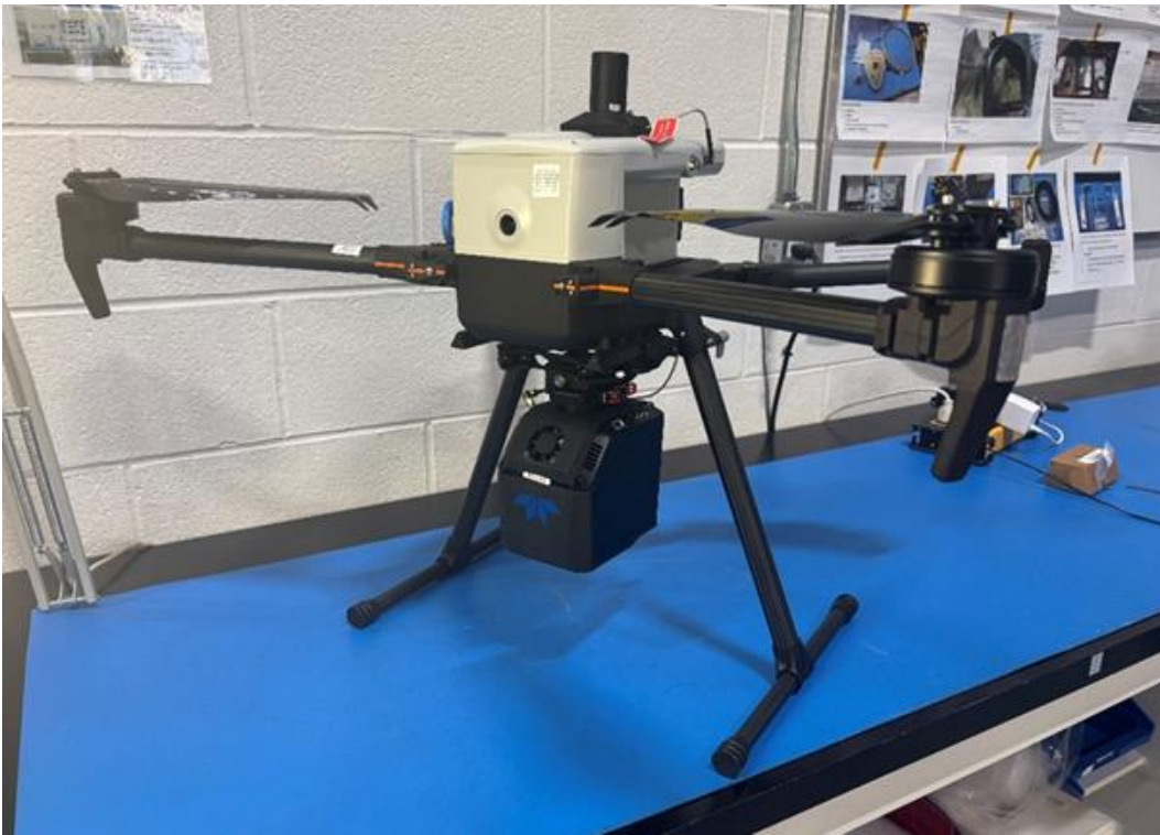
Figure 5-15: EchoONE and IF800 final setup
