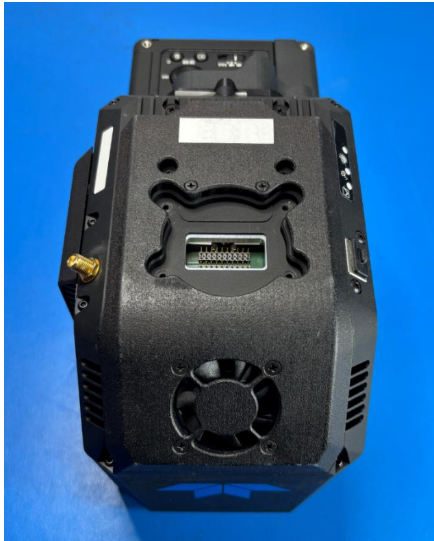
Figure 2-5: EchoONE sensor with covers removed
