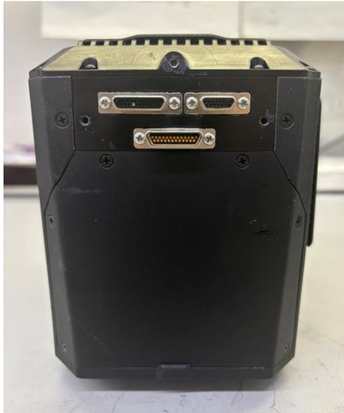
Figure 2-9: Connectors on back of EchoONE sensor
