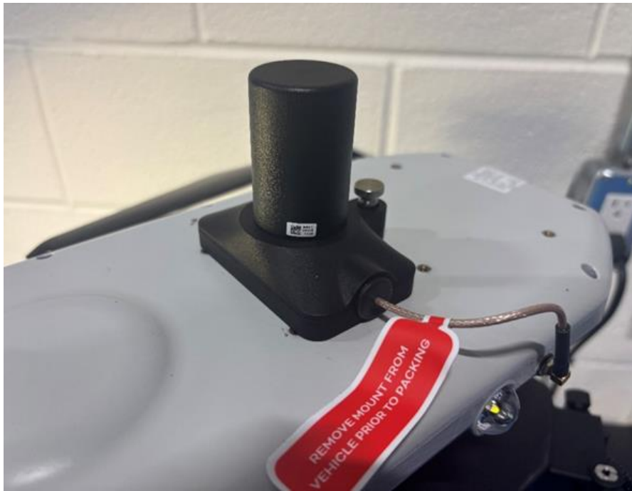
Figure 5-10: GNSS mount on the IF800
