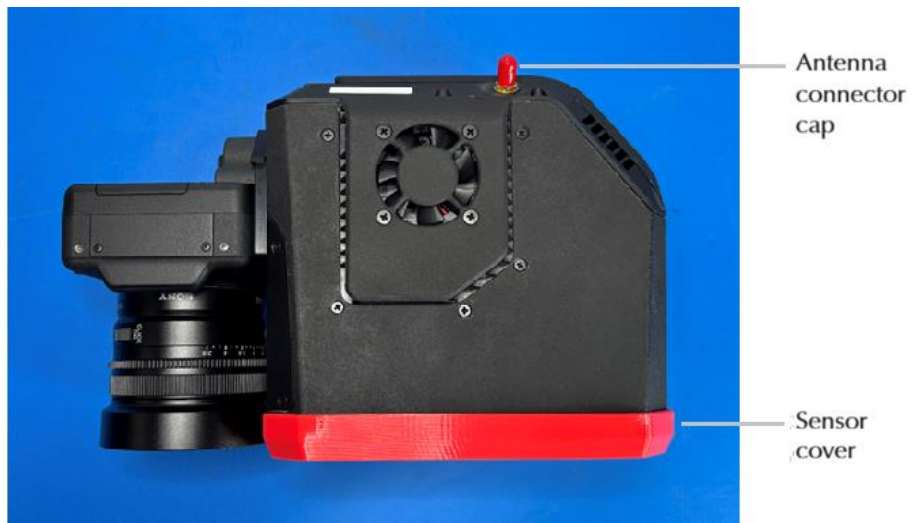
Figure 2-4: Antenna connector cap and sensor cover
