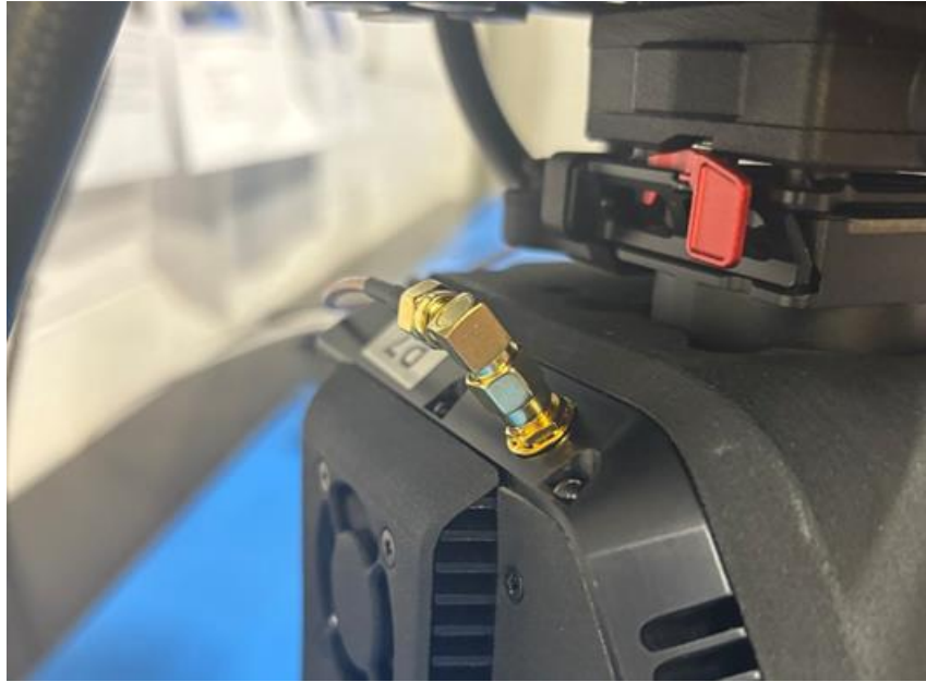
Figure 5-14: GNSS cable connected to the EchoONE
