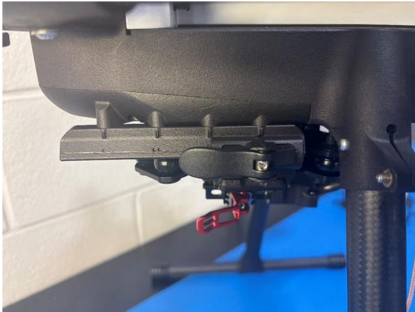
Figure 5-9: Damping plate on the IF800
